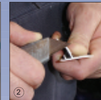
2 Carefully remove frays left by saw cut!
